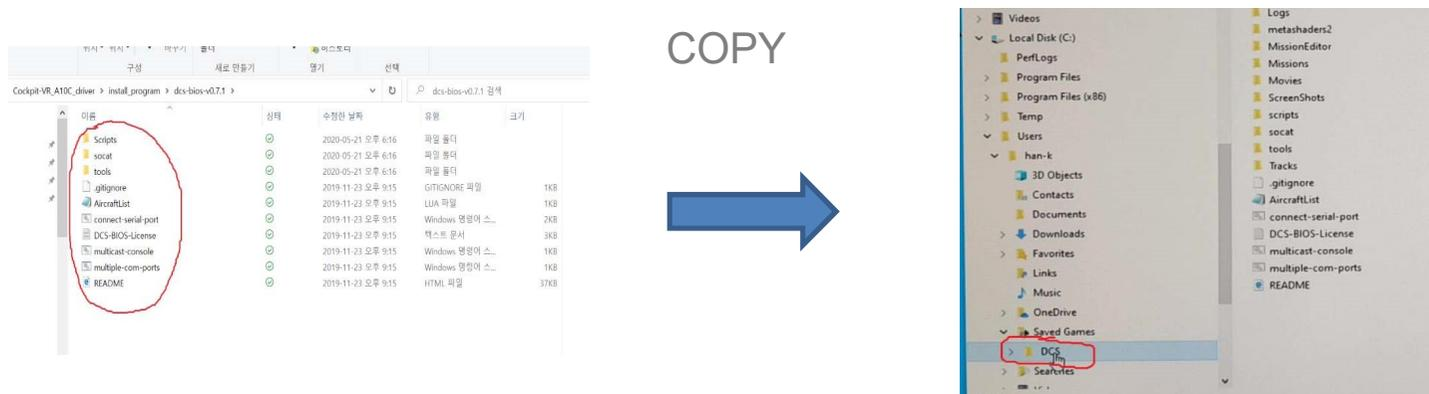
Copy all files and folders inside the Dcs-bios-v0.7.1 folder to the DCS folder on the C: drive.
